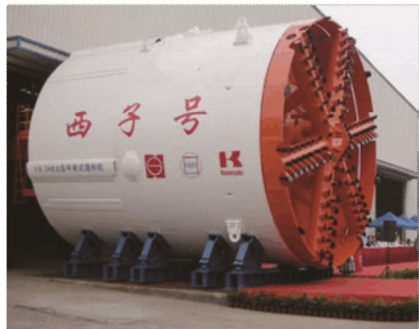
Fig. 1. Shield tunneling machine
